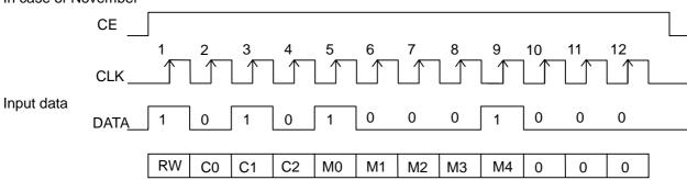
(Note3) In case of over than 12 bits data, valid data is the first 4 bits as System control data and the last 8 bits as Timer data. (In case of Days of week, it is the last 4 bits is effective.)
